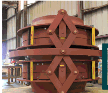
42" Dia. Hinged Universal Expansion Joint Designed with Panto-graphic Linkage
