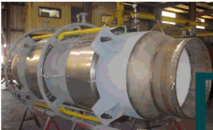
Universal Expansion Joint with 5" Thick Refractory Lining for a Styrene Plant
