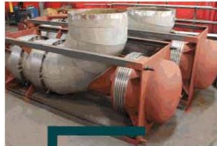
32" Dia. Elbow Pressure Balanced Expansion Joint for an Exhaust Duct in a Power Plant
