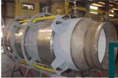
Universal Expansion Joint with 5" Thick Refractory Lining for a Styrene Plant
