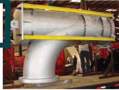
36" Pressure Balanced Elbow Expansion Joint with Inconel 625 LCF Bellows
